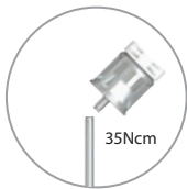
Handle neck is designed to be broke in 35Ncm for prevent hex tip fracture
